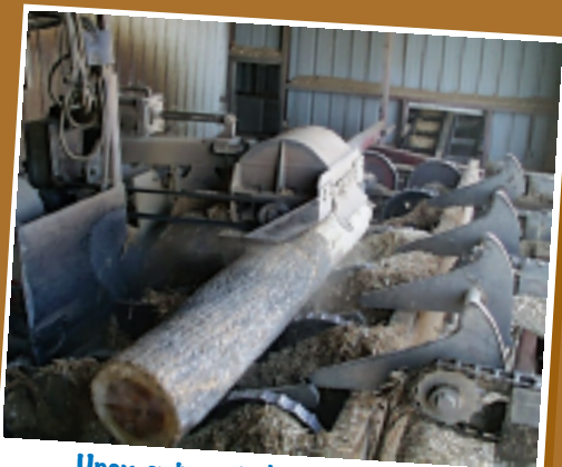
Upon entry at the mill, the bark is removed from the logs.
